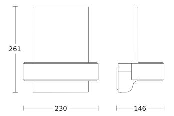
Possible mounting height: 1,80 m - 2,50 m Orange: radial and tangential
